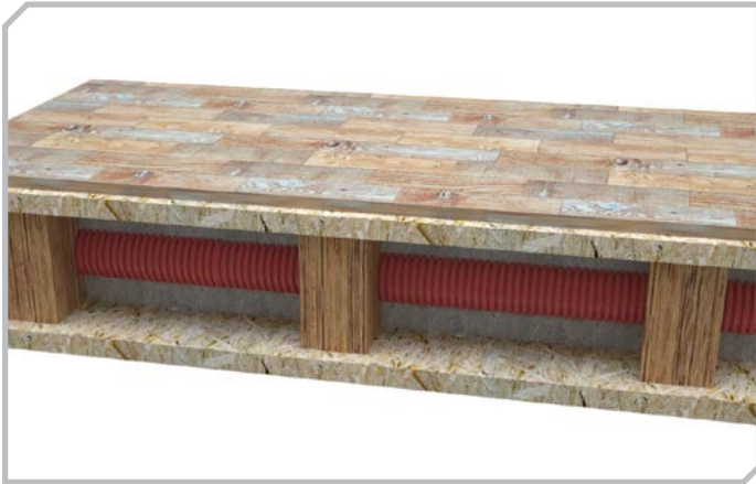
Inside wooden floor structures through the beams
